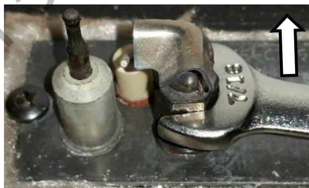
Figure 26 – Pilot in NG (Pilot Gate forward)
