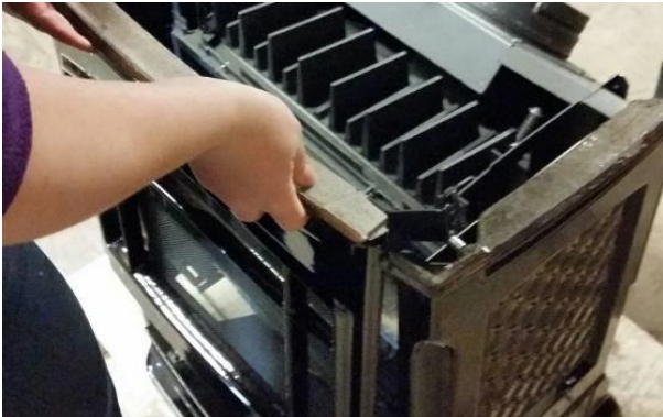
Figure 3 – Front Panel Removal
