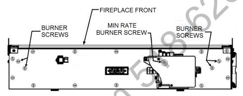
Location of the burner mounting screws looking up at the underside of the fireplace.
