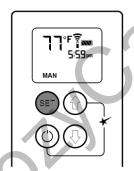
In MAN mode, flame height is controlled by the up and down arrows. HO and LO commands function but otherwise is a "more or less flame" mode only.
