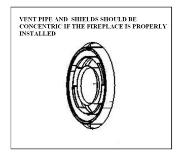
quite heavy. Lift the fireplace up and guide the vent pipe into the vent pipe opening in the mounting plate. The vent pipe must be at the highest location possible in the vent pipe opening (almost touching the inner vent pipe heat shield) to allow the mounting tabs on the rear of the fireplace to clear the top of the mounting brackets on the mounting plate. Refer to the adjacent illustration.
