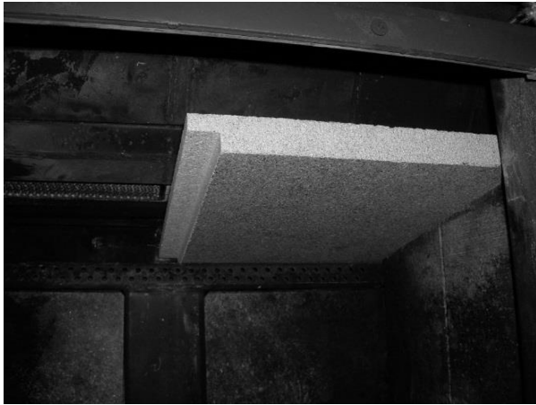
Figure 20 (cont.) - Removing/Replacing the Baffle for Inspection
