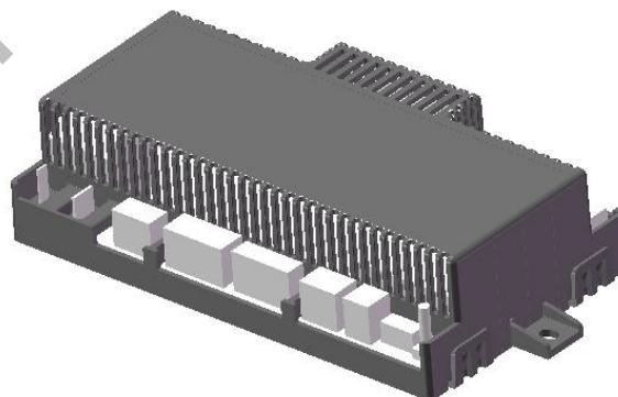
Figure 5 – Proflame 2 Control Board
