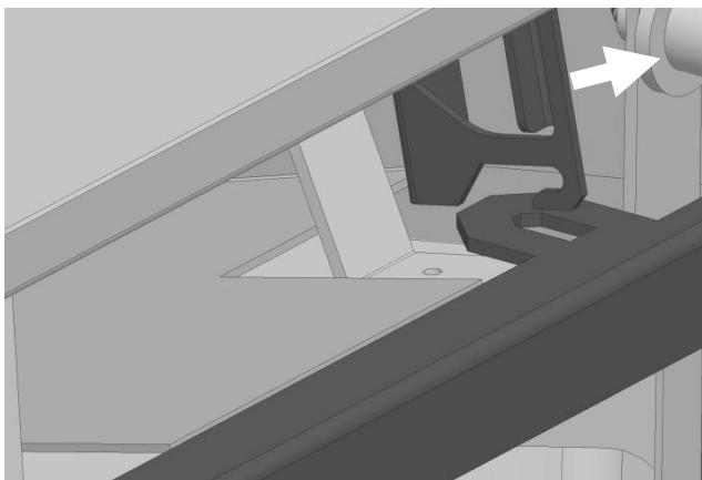
Figure 12 – Glass Frame Upper Mounting Detail
