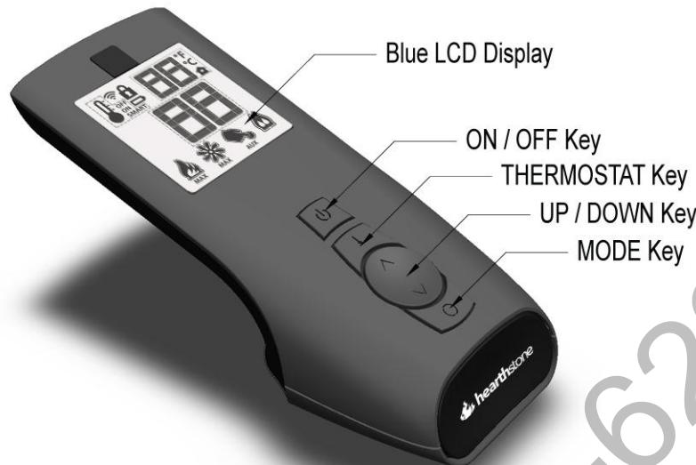
**Figure 9 - Remote Transmitter Function Keys** (remote color may differ from shown)
