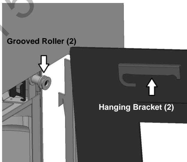
Figure 30 – Façade Mounting Point Detail
