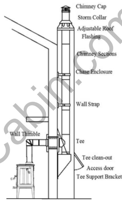
Chimney through outer wall with enclosed chase.
