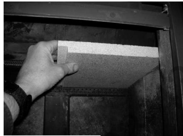
**Figure 19b – Removing / Replacing the Baffle**
