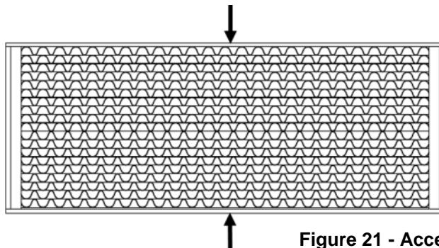
Figure 21 - Acceptable Catalytic Distortion
