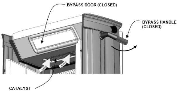
Figure 9 – Bypass Closed
