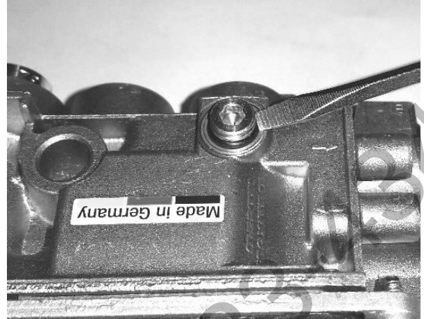
Figure 24 – Low Flow Orifice Removal – O-ring
