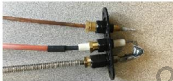
Pilot Mechanism Re-assembled
