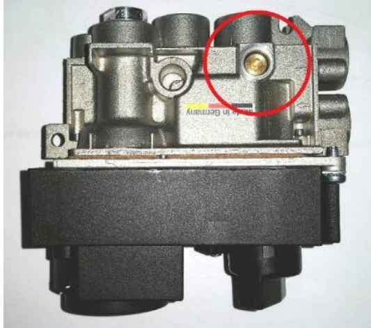
Figure 20 – Low Flow Orifice Location
