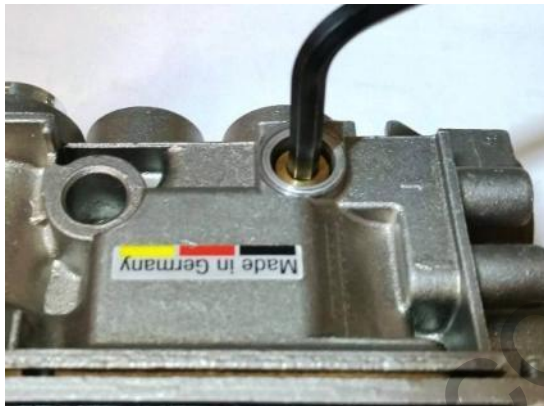
Figure 21 – Low Flow Orifice Removal
