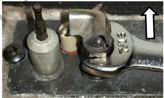
Figure 26 – Pilot in NG (Pilot Gate forward)
