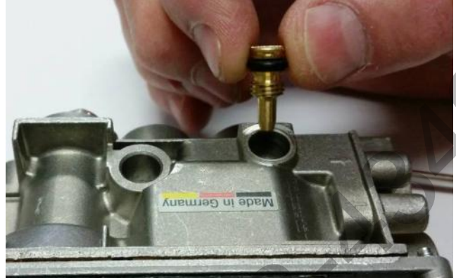
Figure 23 – NG Low Flow Screw Removal
