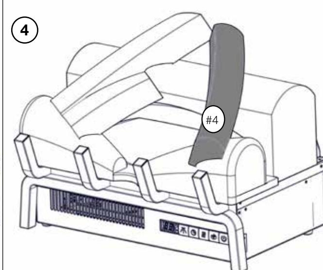
Place log (#4) into the groove. Ensure the log is secure, as shown.
