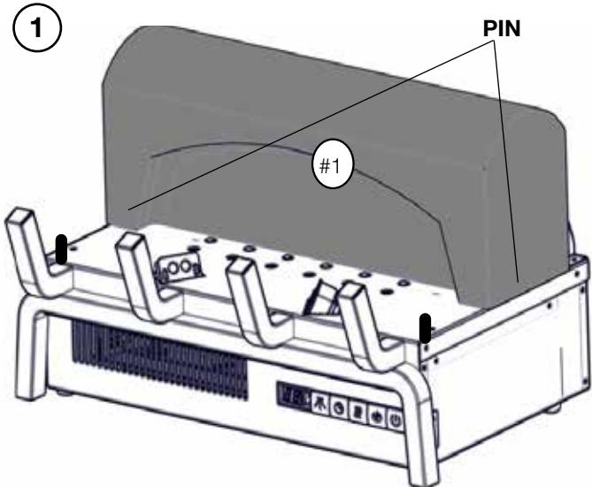
Place the log (#1) onto the pins. Ensure the log is secure onto the pins, as shown.
