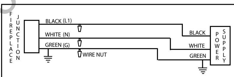
**NOTE:** To aid with moving the appliance, leave enough wire so that the log set can be removed from the enclosure without disconnecting the power supply. If servicing, shut off power supply.
