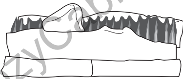
Figure 37 - Correct Front Burner Flame Pattern
