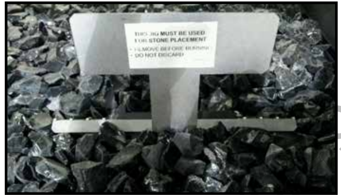
Figure 9.7 Rock Placement Jig
