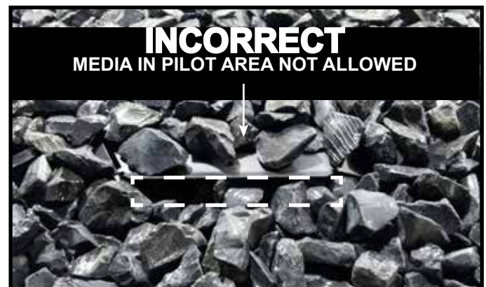
Figure 9.9 INCORRECT Media Placement
