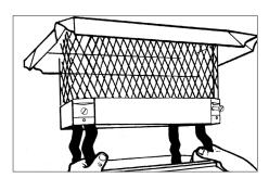
2. Insert two (2) legs into the liner no more than 1". By exerting pressure as shown, force the other legs inside the liner. Push cover straight down into the chimney liner as far as possible. Tighten the screws on all four (4) legs until the cover is held firmly into the flue tile.
