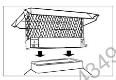
2. Place the chimney cover on the flue liner and align the base with the flue liner. Partially tighten each of the four screws until they are snug to the liner. Then tighten each of the four screws firmly to the liner.
