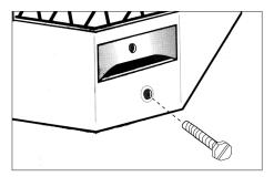
1. Insert one screw into the lower hole located in each mitered corner of the chimney cover band. (Just start the screw into the hole a few turns, until all four screws are started.)
