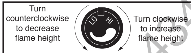
Fig. 20 Flame adjustment knob for Honeywell Valve.
