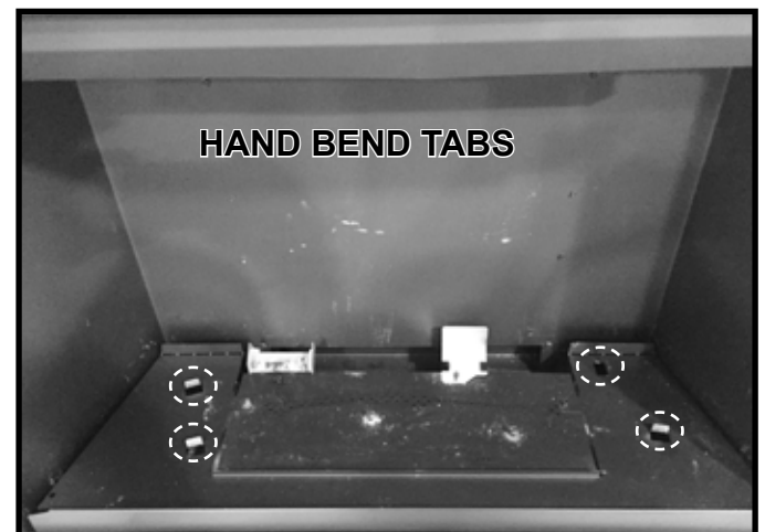
Figure 3. Hand Bend Tab Locations - QUARTZ36 Shown
