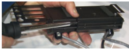
Secure the 2 boxes together with one screw.
