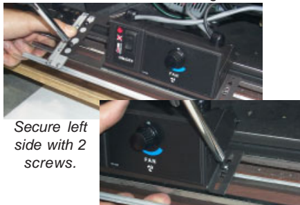
Secure right side with one screw.
