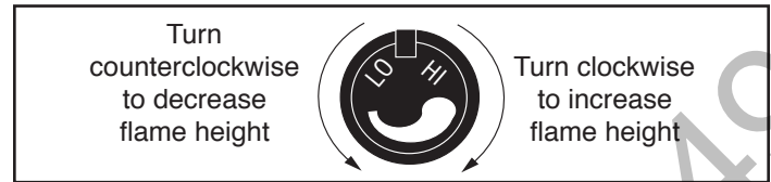
Figure 47 - Flame adjustment knob for Honeywell valve.
