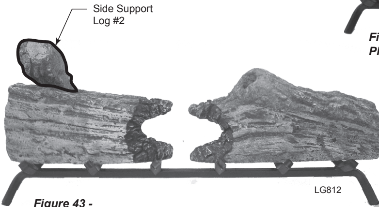
Figure 43 - Place Side Support Log #2 on Top Left of Log #1a
