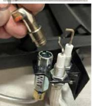
Locate pilot orifice screw, remove using flat head screwdriver. Replace with LP screw and re-install.
