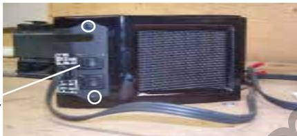
Fan Switch Plate Assembly
