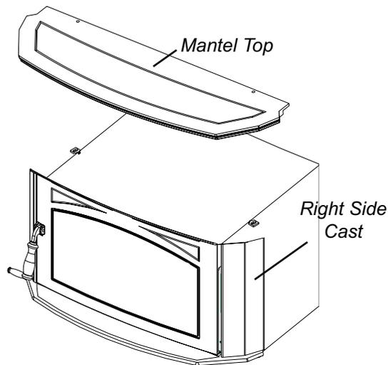
With the Mantel Top in place check to make sure there is no gap between the nut retainer and the underside cast of the Mantel Top. If there is a gap present you will need to lower that side cast by loosening 2 bolts, see step 6 for bolt location (check to see if level).
