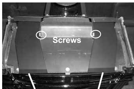
Left Side Air Channel
