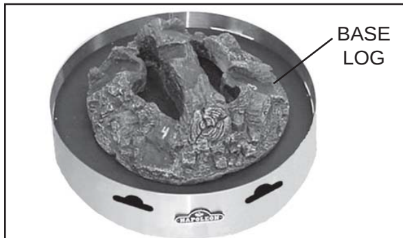
4.1.1 Set base log onto burner ensuring stud and bracket fit into hole and notch. Base log should sit flat on "Patioflame" base.
