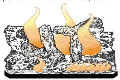
3/8" - 1/2" FLAME MUST ENVELOPE UPPER 3/8" TO 1/2" OF THERMOCOUPLE & THERMOPILE
