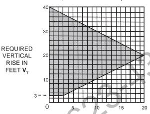
HORIZONTAL VENT RUN PLUS OFFSET IN FEET H, The shaded area within the lines represents acceptable values for H, and V,
