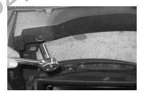
Remove the right interior side brick held in by a bracket on the top of the brick. Take out the hex head bolt and remove the bracket and slide the brick out.
