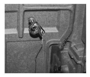
6. Locate the primary air frame and valve in the rear bottom of the stove. It is oriented on a 45° angle.
