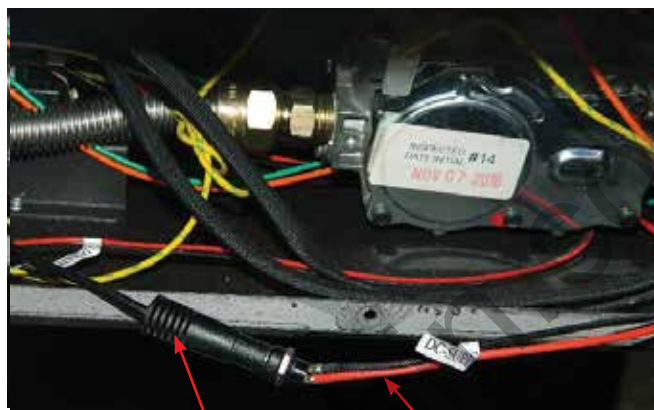
DC supply wire from wiring harness
