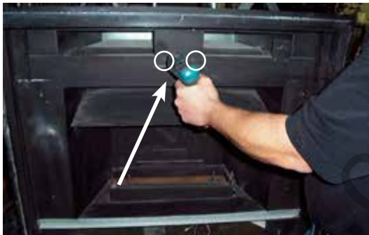
Remove 2 screws - remove Top Bracket
