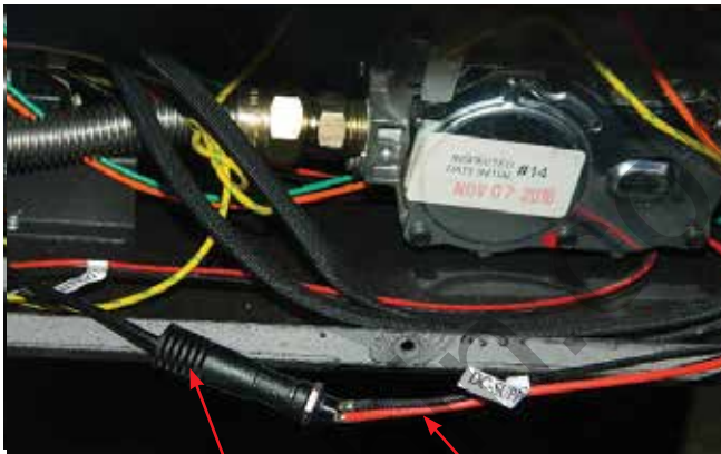
DC supply wire from wiring harness
