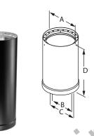
Designed for installation with minimum clearance to combustibles (6" to walls, 8" from top of horizontal run to ceiling). Available in 6", 7", and 8" diameters. Subtract 3/4" for installed length. Constructed with a stainless steel inner wall.
