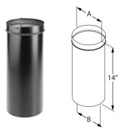
Use to adapt DuraBlack pipe to ceiling support box or finishing collar. Adds 3" - 13" of length to rigid pipe. Allows drip-free installation without cutting the pipe. Can be used in line to create a telescoping combination when used with a straight length of pipe. Requires screws.
