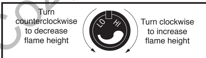
Fig. 51 Flame adjustment knob for Honeywell valve.
