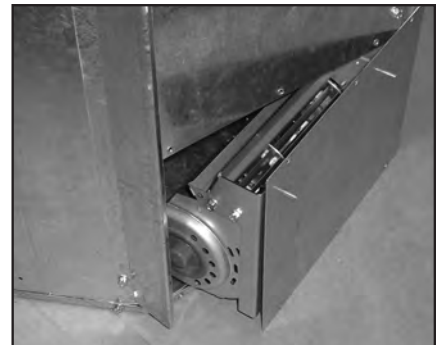
Figure 53: Installing Fan Through the Back.
