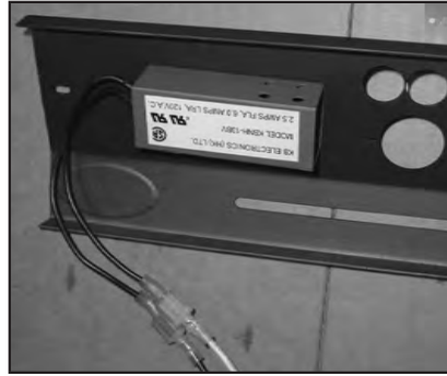
Figure 49. Install Fan Controller.
