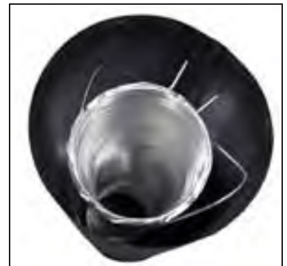
Figure 27: Wire Spacer in Place.
