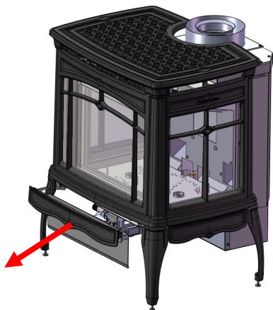
Figure 28 - Remove Cast Cover
