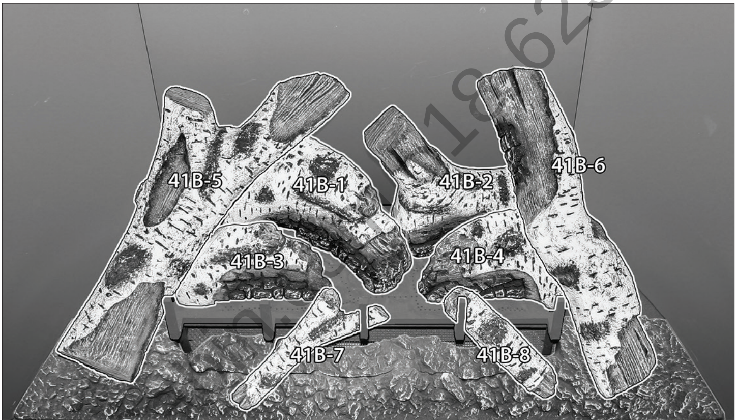
Figure 1, #B41-B501 Log Set Installation
