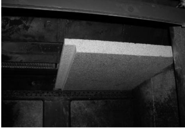
Figure 16 (cont.) - Removing/Replacing the Baffle for Inspection
