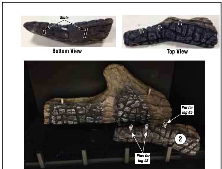
Figure 42 - Install bottom right log (2)
