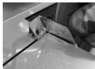
Step 1: Carefully bend up the two (2) tabs on the heat shield at a 90° angle from each opposite joint and then the foot of the Standoff at approximately a 45° angle.
