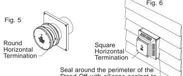
Stand Off with silicone sealant to ensure a weather tight seal
