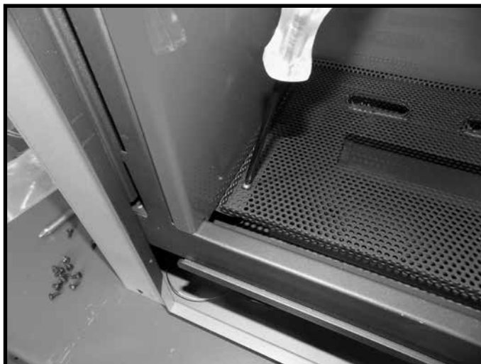
Figure 46: Securing glass media tray to firebox floor.
